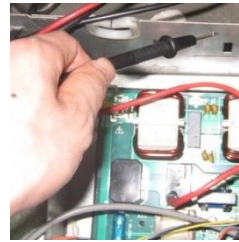
Figure 2: Measuring resistances between compressor terminals and ground
