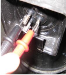
Figure 1: Measuring resistances among compressor terminals
