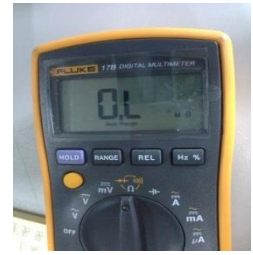
Figure 2: Measuring resistances between compressor terminals and ground
