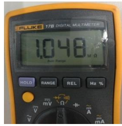
Figure 1: Measuring resistances among compressor terminals
